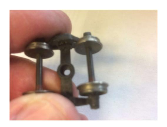
So I popped off both axles carefully, and inspected the equipment, specifically the journals and axles.
