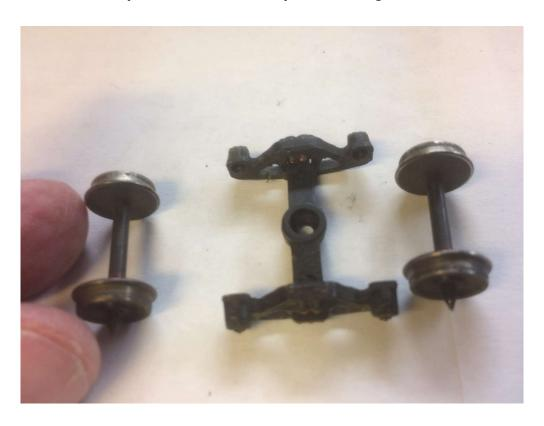
I found dirt in two journals and a small burr. Be sure to remove all dirt and burrs. Our objective is to minimize friction.
