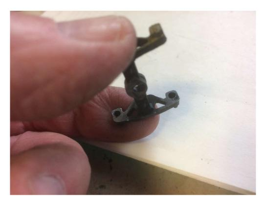
Take note that axles are insulated. They go on the same side. Reassemble making sure the axles spin freely and the springs are in proper position.
